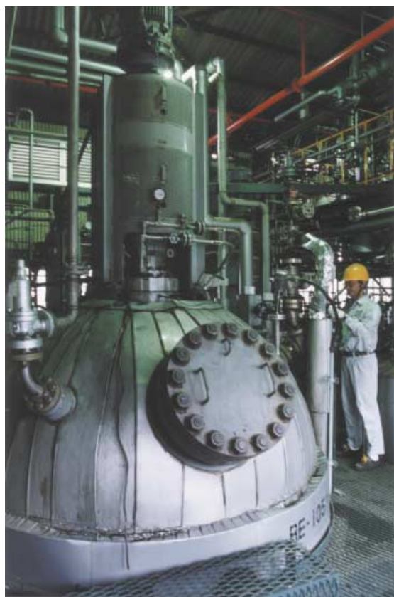
Figure 7. A large-scale BINAP-Ru-catalyzed hydrogenation at Takasago International Co.
